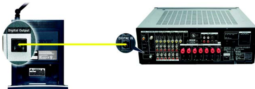
Figure 5-8: Connecting the Optical Cable to Your Stereo
